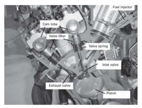
Figure 5.1: DOHC type valve system.
