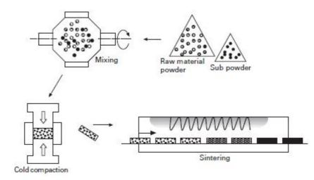
Figure 5.15: Powder metallurgical process.
