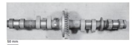
Figure 5.4: Camshaft installing a drive sprocket at the center
