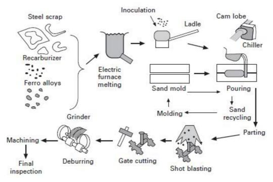
Figure 5.10: Casting process.
