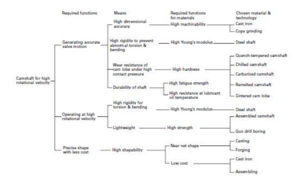
Figure 5.5: Functions of camshafts for high rotational velocity
