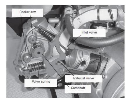
Figure 5.3: SOHC type valve system installing twin rocker arms.
