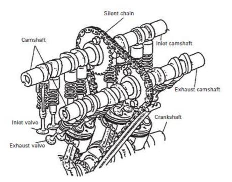
Figure 5.2: Schematic illustration of a valve train
